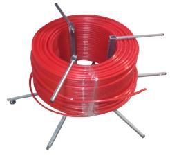
A pipe coil is placed on a decoiler allowing simple pipe uncoiling while subsequent pipe sections are laid
